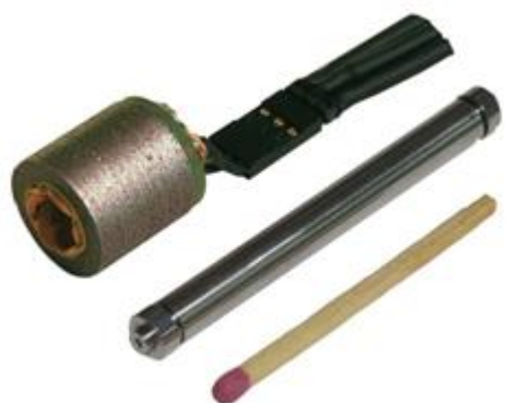
Fig. 4. Photograph of the stator and rotor of the drive system. The extra long titanium rotor, containing two magnets, is used for a motor-generator test bench. A high-speed ball bearing is mounted on each end of the rotor.
